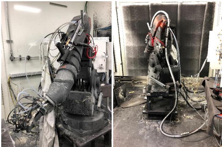
Figure 9: Recorable Coax System in Place on Robot
