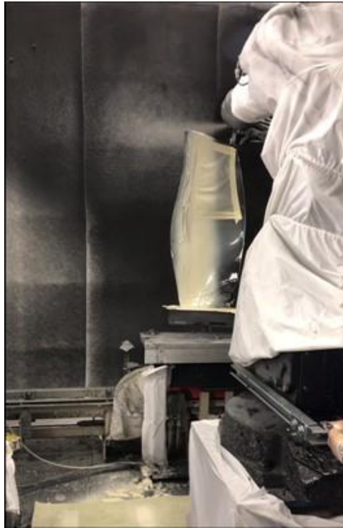
Figure 4: Conveyorized Robotic Paint Application
