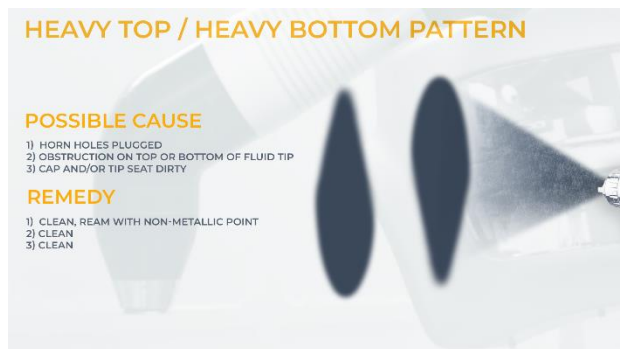
Figure 18: SprayVision Troubleshooting Guide for Pattern Distribution
