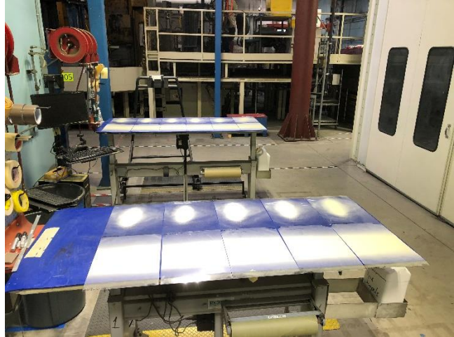
Figure 12: Set of 11 Static and 11 Dynamic Films to Analyze Viscosity Impact on Painting Process
