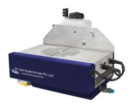
foundation of the system the Temperature Control Unit. Using Peltier technology, the unit material senses temperature and either adds or removes heat to ensure consistent material temperature. The unit is very small and can mount directly on the machine, or sit on a tabletop if necessary.
