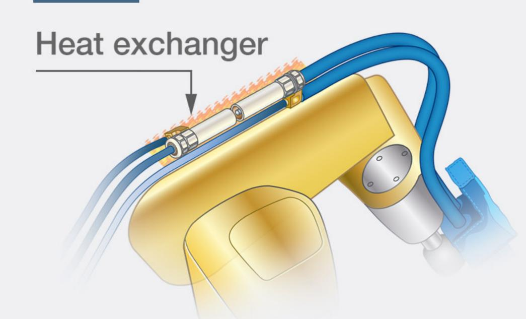
Heat exchangers and thermal sizing tools are some of the most efficient devices available for addressing thermal loads in any dispense system. These solutions can be modified to meet the requirements and specifications of various dispense systems.
